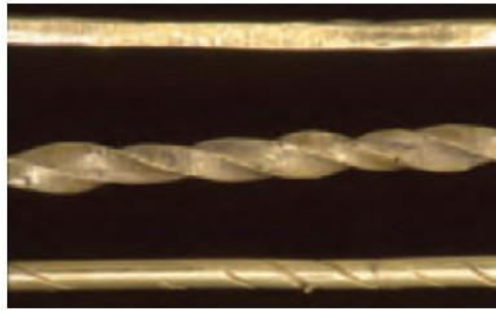
Figure 10: Block twisted wire (after Craddock 2009, Fig. 15.5).
