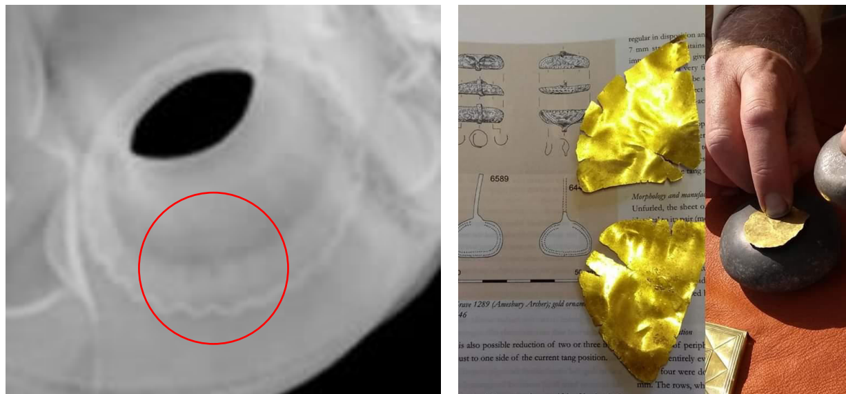
Figure 17: Left: the cracks visible on the x-radiograph and, right, the cracked sheet margin of gold that has not been fully annealed (heated) before working (Image © Sally & Gareth Riseborough)
