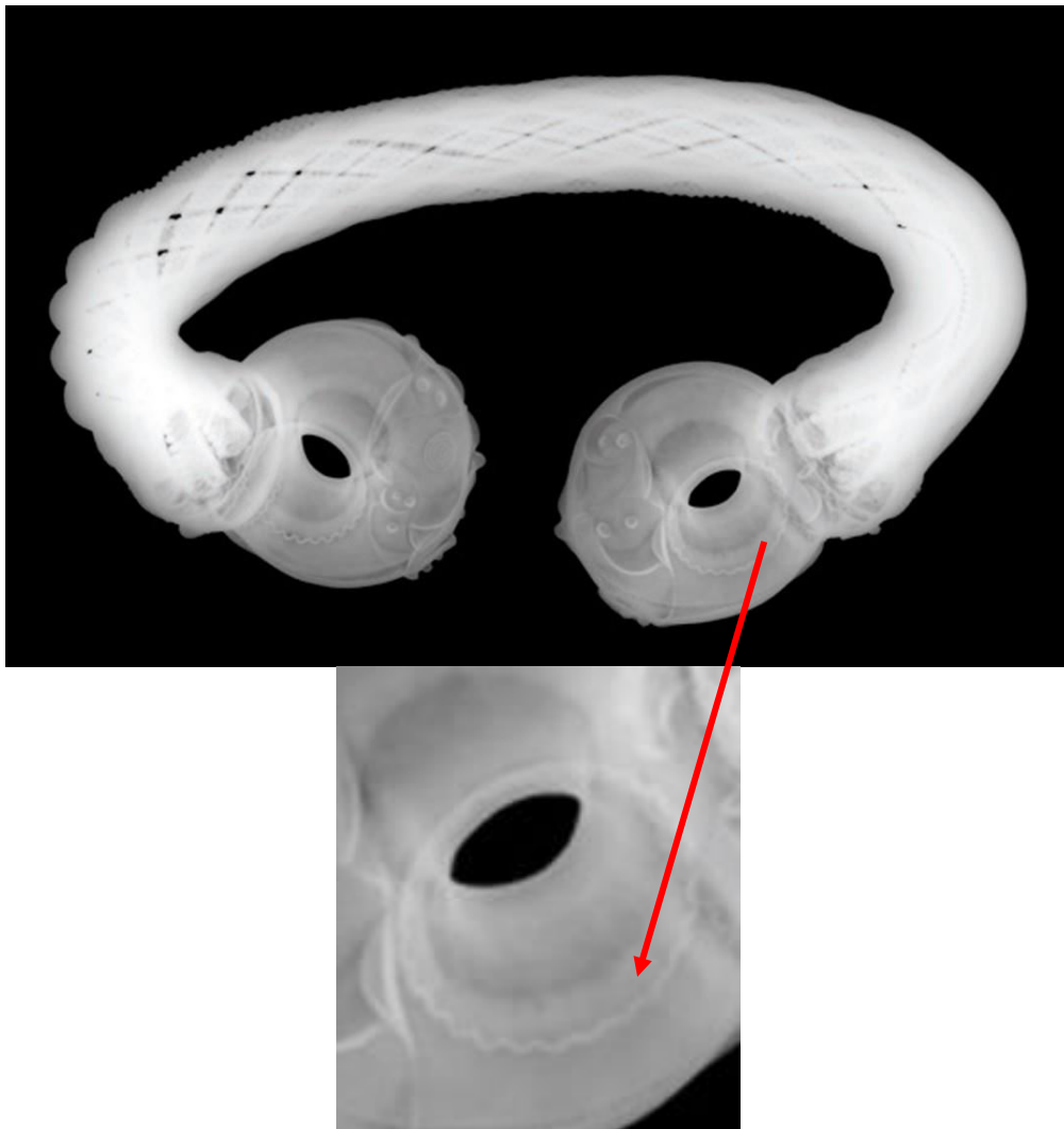
Figure 15: The x-radiograph of the Snettisham Great torc, close up shows the overlapping seam and 'splay' (from Flynn 2017, Image © The trustees of the British Museum)
