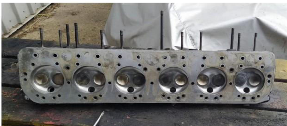
Figure 14: Inlet and exhaust valves fitted in a 20/25 cylinder head (Image © Hamish McNaught)
