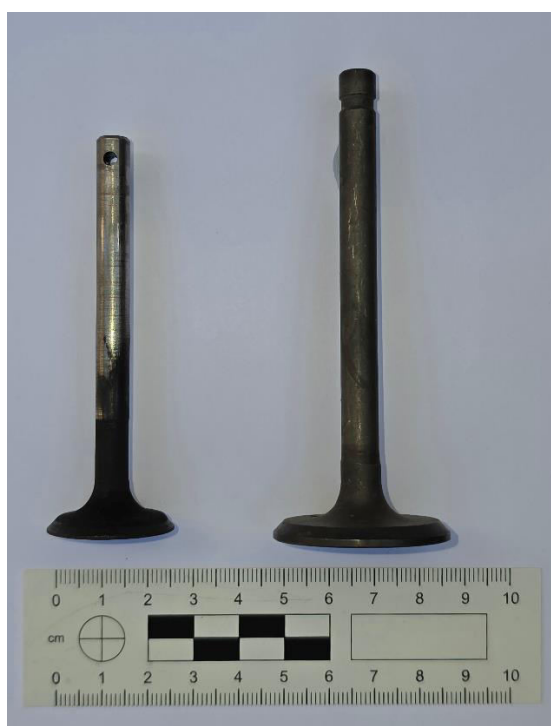
Figure 15: Valves from an Austin 7 (left) and Ford 1500 pre-crossflow (right) (Image © Tess Machling)
